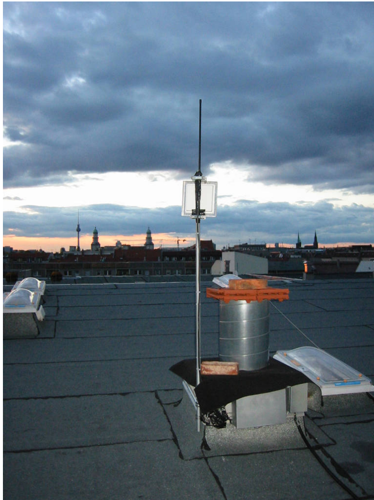
Figure 13.3: One of the first Freifunk nodes setup with a white patch sector antenna for remote connection and a black omnidirectional antenna on top of it to offer local service.
